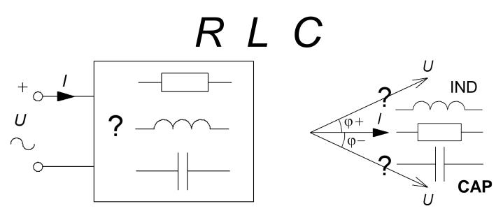
In general, our circuits are a mixture of different R L and C. The phase between I and U is then not  $\pm 90^{\circ}$  but can have any intermediate value. Positive phase means that the inductances dominates over capacitances, we have inductive character **IND**. Negative phase means that the capacitance dominates over the inductances, we have capacitive character **CAP**.
