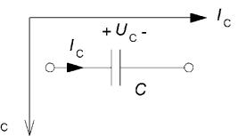
The method with complex pointer *automatically* keeps track of the phase angles if we consider the capacitor reactance  $X_{\rm C}$ as **negative**, and hence the inductor reactance  $X_{\rm L}$  as **positive**.
