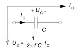
Phasor  $U_{\rm C}$  is  $I_{\rm C}/(\omega C)$  and it lags 90° *after*  $I_{\rm C}$ . The entity  $1/(\omega C)$  is the "amount" of the capacitor's AC resistance, **reactance**  $X_{\rm C}$  [ $\Omega$ ].
