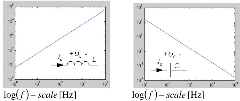
Often electronics engineers use log-log scale. The inductor and capacitor reactances will then both be "linear" relationship in such charts.
