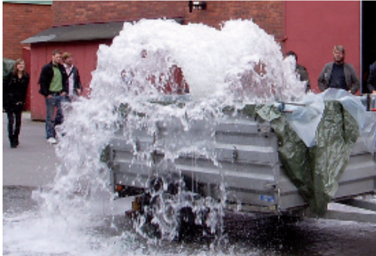
Flood pump (120 litres/s) developed by students, Integrated Product Development. Photo: Lars Hagman
