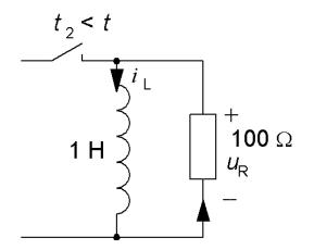
When the voltage source 10 V is disconnected, the current is driven by the inductor. The voltage drop over the 100  $\Omega$ resistor  $U_R$  at first is  $-100 \cdot 0,1 = -10$  V. The minus sign comes from the fact that the current is entering the resistor in the part of the resistor we defined negative.
