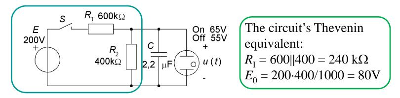
The capacitor is charged from 0V up to 80V at 65V the neon lamp lights up (and discharges the capacitor to 55V when it goes off).
