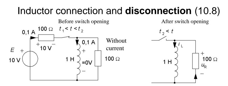
After  $t_2$  the current starts from the "same value" 0,1 A ( $i_0$ ) as before the switch opening, and then the current will decrease down to 0 ( $i_{\infty}$ ). Time constant will be  $\tau = L/R = 1/100 = 0,01$  s.
