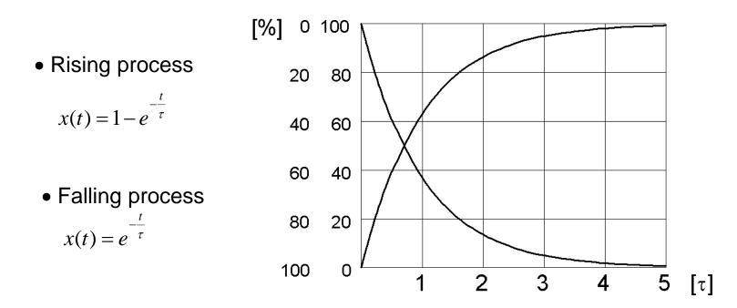
The Quick Formula directly provides the equation for a rising/falling <u>ex</u>ponential process:
