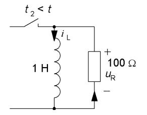
When the voltage source 10 V is disconnected, the current is driven by the inductor. The voltage drop over the 100  $\Omega$ resistor  $U_{\rm R}$  at first is  $-100 \cdot 0,1 = -10$  V. The minus sign comes from the fact that the current is entering the resistor in the part of the resistor we defined negative.
