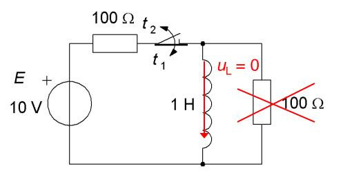
b) How large is the current through the inductor after a long time interval?  $E + 10 V \qquad 1 H$
