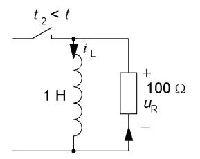
When the voltage source 10 V is disconnected, the current is driven by the inductor. The voltage drop over the 100  $\Omega$ resistor  $U_R$  at first is  $\bigcirc 100.0,1 = -10$  V. The minus sign comes from the fact that the current is entering the resistor in the part of the resistor we defined negative.
