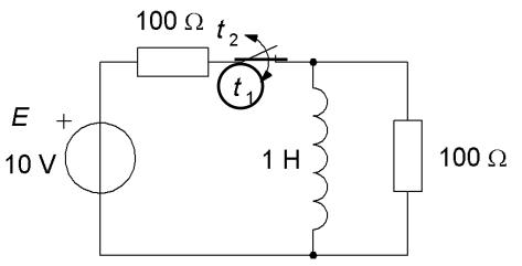
*E* is a DC source. At the time  $t_1$  the switch is closed.
