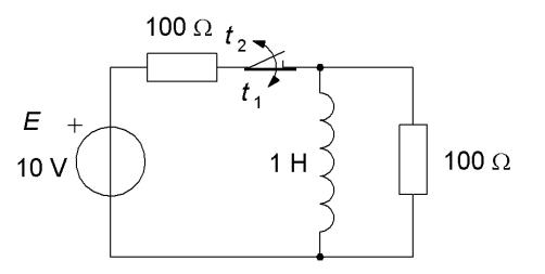
b) How large is the current through the inductor after a long time interval?
