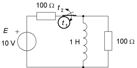
Answer: The inductor has has "current inertia". The first moment  $(t_1)$  the current will be the "same" i = 0.
