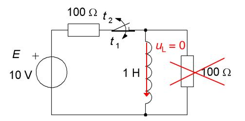
Answer: After a long time, the changes have faded away. The voltage across the inductor (is due to changes) then is 0, the inductor is "shorting" the 100  $\Omega$  parallel resistor. The 100  $\Omega$  series resistor limits the current from the voltage source.  $i = 10V/100\Omega = 0,1$  A.
