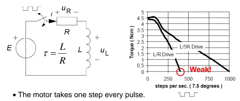
The faster you drive, the shorter the pulses. Due to the **time constant**  $\tau$  do not have time to reach the peak current in the windings and the motor becomes weak.
