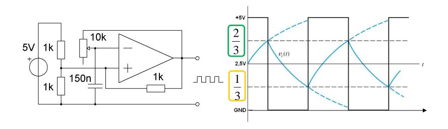
The comparator charges the capacitor to the upper trigger level, then it turns the output on and discharges the capacitor to the lower trigger level. The frequency of the output of the comparator depends on the product  $R \cdot C$ . Since *C* is constant so will the *R* controls the frequency.
