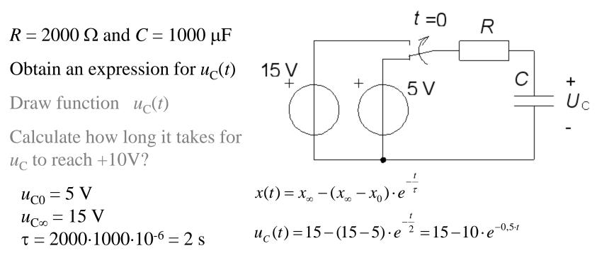
**Note:** Capacitor voltage is continuous – If you put a voltage across a capacitor it can not charge instantaneously (would require infinite current). The voltage will not change at once.
