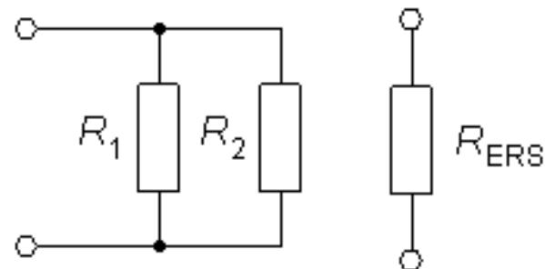
$$\frac{1}{R_{\text{ERS}}} = \frac{1}{R_1} + \frac{1}{R_2} = \frac{R_2}{R_2} \cdot \frac{1}{R_1} + \frac{R_1}{R_1} \cdot \frac{1}{R_2} = \frac{R_1 + R_2}{R_1 \cdot R_2}$$
