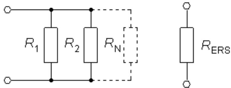
$$R_1 = R_2 = \dots = R_N = R$$
