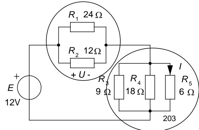
$$R_{1//2} = \frac{24 \cdot 12}{24 + 12} = 8 \quad \frac{1}{R_{3//4//5}} = \frac{1}{9} + \frac{1}{18} + \frac{1}{6} = \frac{2+1+3}{18} = \frac{6}{18} \Rightarrow R_{3//4//5} = \frac{18}{6} = 3$$
