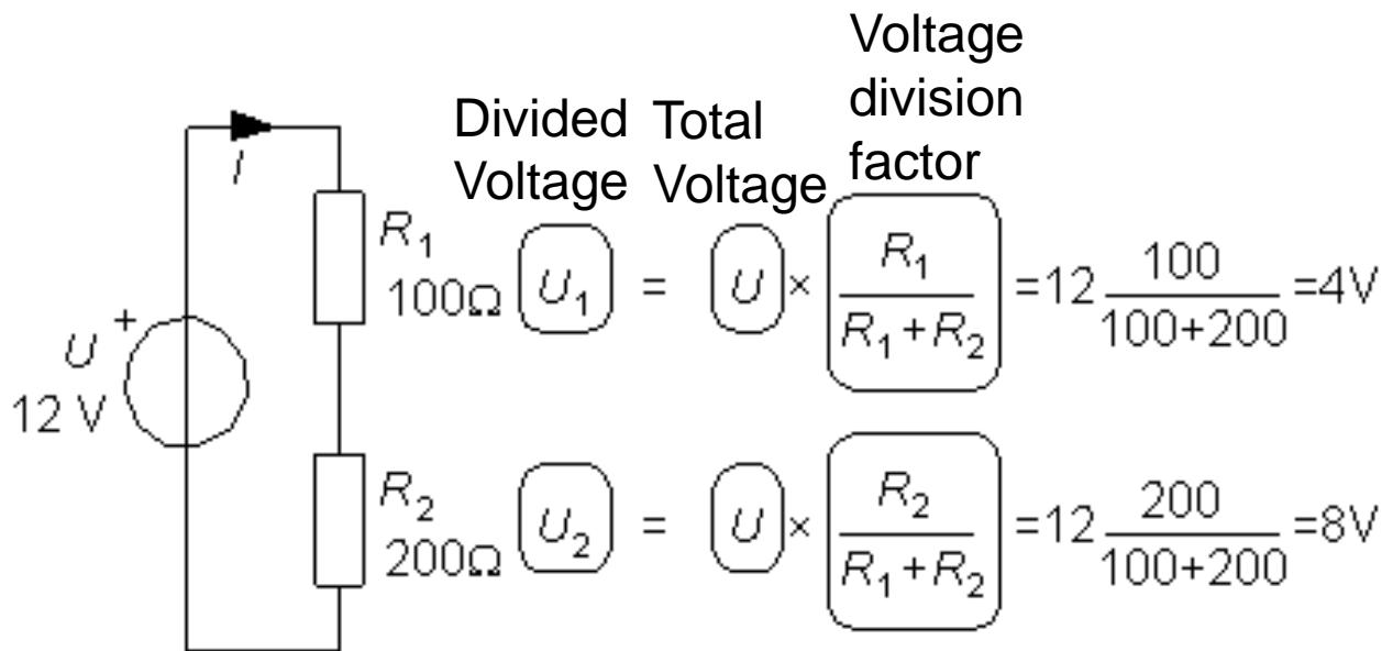
According to the voltage divider formula you get a divided voltage, for example  $U_1$  across the resistor  $R_1$ , by multiplying the total voltage  $U$  with a voltage division factor. This voltage division factor is the resistance  $R_1$  divided by the sum of all the resistors that are in the series connection.
