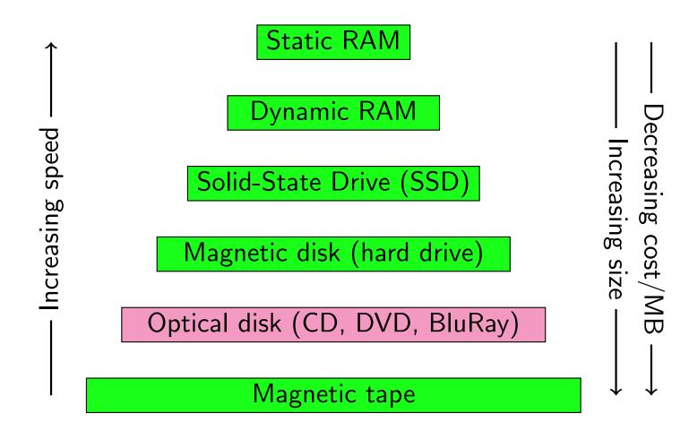
Optical disk storage is marked with a special color because it does not respect the size hierarchy.
