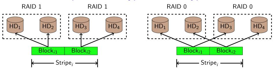
Failure of a single drive: Always tolerated in both configurations.
