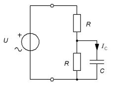
$\frac{\underline{I}_{C}}{\underline{U}} = \frac{j\omega C}{2 + j\omega RC} \qquad \omega RC = 2 \quad \Rightarrow \qquad f_{G} = \frac{1}{2\pi} \cdot \frac{2}{RC}$  $\frac{\underline{I}_{C}}{\underline{U}} = \frac{j\omega C}{2 + j\omega RC} = \frac{j\frac{2}{R}}{2 + j2} \quad \Rightarrow \quad \frac{I_{C}}{U} = \frac{\frac{2}{R}}{\sqrt{2^{2} + 2^{2}}} = \frac{1}{R \cdot \sqrt{2}}$
