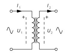
Calculate the two values that are missing.  $I_1$  and  $U_2$ .
