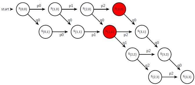
If we cannot find a path from the initial state to the final state without reaching a state for which a predicate is true then the predicate is *definitely true* during the execution.
