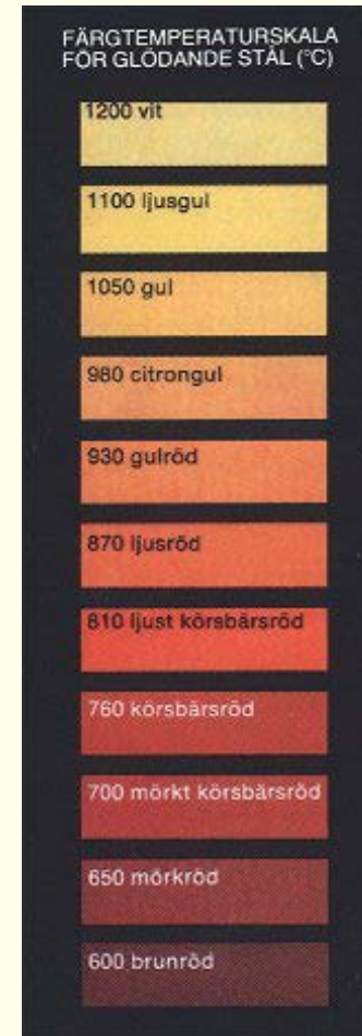
Chart to estimate steel temperature in steelworks.
