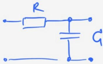
Fourier (no transient effect)  $\leadsto$  Transformed Circuit
