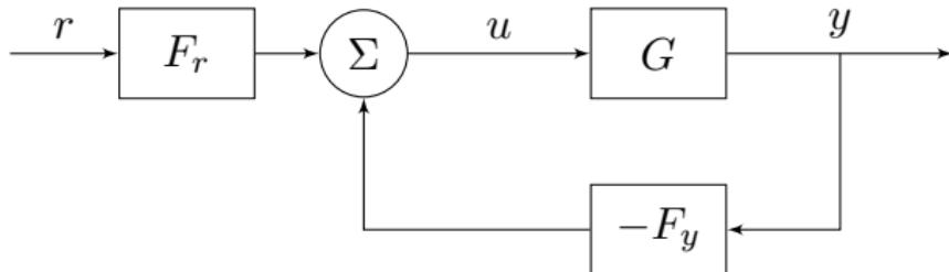
$$\begin{aligned} F_r &= \left( 1 - L[sI - (A - BL - KC)]^{-1}B \right) l_0 \\ F_y &= L[sI - (A - BL - KC)]^{-1}K \end{aligned}$$
