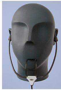
Figure 2.3. The Sennheiser MK2002 binaural microphones used in the study. (Literaturcafe, 2013)
