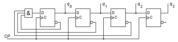
**a)** (2p) Analyze the sequential circuits in the figure and draw the **full state diagram** and the **full state table**. If the counter would start in any other state than any of the four desired "one hot" states, how many clock pulses are required, in the worst case, before the counter has "corrected" this and ends up in the correct sequence?
