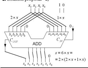
b) The greatest number will be  $s_{\text{max}} = 6.15 = 90$ . Since the calculator is not allowed at the exam, this time we can choose to transform 90 to at **binary number** in the same way as in a)
