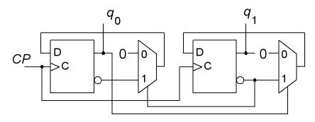
Sequential circuit shown above starts in the state  $q_1q_0\,$  00. Analyze the circuit and give the sequence of its states for the following four clock pulses.
