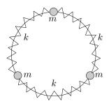
**Problem 1.** Three equal particles of mass m are sliding on a smooth, horizontal, circular ring. Three equal linear thin springs with spring constant k are also threaded on the ring, connecting the particles. Formulate the normal mode equations as an eigenvalue problem, and in particular find the angular frequencies of the oscillating modes, and the mode shape for the non-oscillating mode.
