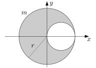
**Problem 4.** From a thin, homogeneous, circular plate of mass m and radius r, a circular hole of radius r/2 is cut. The hole is tangent to the circumference of the plate. Find the new centre of mass G, and compute the  $3 \times 3$  inertia matrix  $J_G$  for the axes indicated in the figure.
