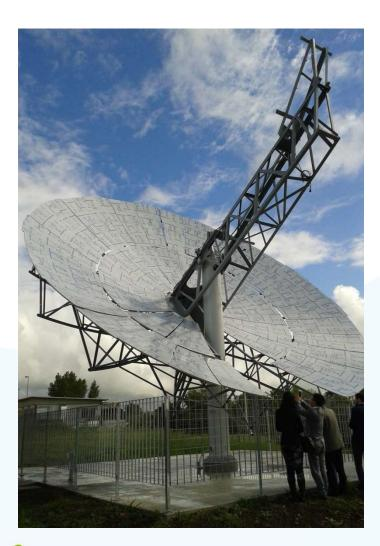
Parabolic mirror for a Concentrated Solar Power (CSP) driven Micro Gas turbine.
