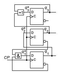
Redesign the circuit, maintaining the function so that it uses **two 2:1 multiplexers** in place of the gates. See figure to the right.
