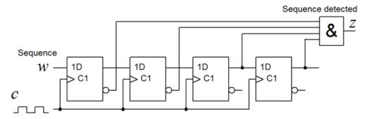
a) (1p) Which bit sequence is detected?
