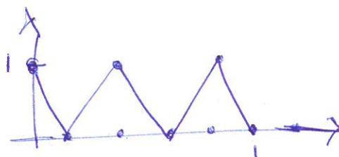
Exact solution :
