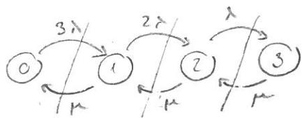
$$\left. \begin{array}{l} p_0 3\lambda = p_1 \mu \\ p_1 2\lambda = p_2 \mu \\ p_2 \lambda = p_3 2\mu \end{array} \right\} \Rightarrow$$
