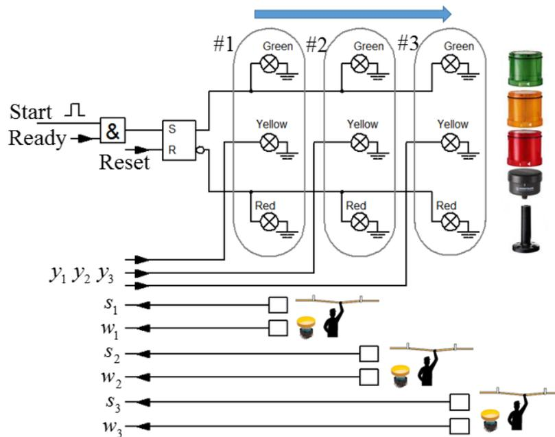
a) ( $a+b=1p$ ) **(Green)** A short pulse  $Start = 1$  can start the assembly line if  $Ready = 1$ . Design a circuit that provides signal  $Ready = 1$  if *none* of the stop signals  $s_1 s_2 s_3$  are 1.
