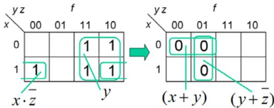
$$f(x, y, z) = \{PoS\}_{\min} = (x + y) \cdot (y + \bar{z})$$
