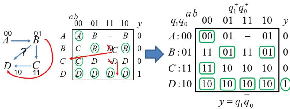
B and D are on Hamming distance 2. For B  $ab = 11$ , unstable state C will forward B to D.
