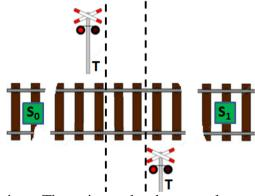
Trains can come from both directions. The train can be shorter or longer than the distance  $S_0$ - $S_1$ . Only one train at a time is passing between  $S_0$  and  $S_1$ .
