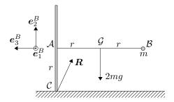
Assuming a horizontal  $\mathcal{AB}$  axis, we can get to any orientation of the body by first doing a simple rotation about a vertical axis to get the desired direction of  $\mathcal{AB}$ , followed by a simple rotation about the  $\mathcal{AB}$  axis to get the desired contact point on the disc. It follows that the angular velocity of the body is the sum of a vertical part and a part parallel to  $\mathcal{AB}$ . Thus
