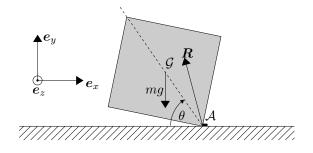
Next study motion after impact. Assuming the corner  $\mathcal{A}$  remains in contact with the stop, which makes it remain an instantaneous centre of rotation, the kinetic energy is
