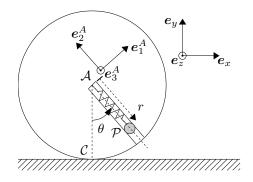
Use the coordinate r of the particle along the tube, and the angle  $\theta$  as generalised coordinates.
