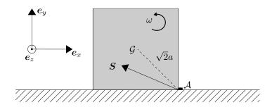
First study the impact. Since the impact impulse S has no moment of force about the point A, the angular momentum about A is unchanged. Before impact we have
