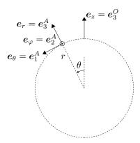
The angular velocity of the first simple rotation is  $\dot{\varphi}e_3^O$  and that of the second is  $\dot{\theta}e_2^A$ , so
