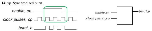
An **asynchronous sequential** circuit has two inputs, *enable en* and *clock pulses cp*. As long as *en* = 1 complete pulses (synchronized with *cp*) should be output as *burst b*. This should happen as fast as a complete pulse (cp = 1) is possible. If *en* gets = 0 during an ongoing pulse then this pulse will also be output completly. The signal *en* is allways longer than the pulse *cp* and the signal *en* will arrive with long intervals. See the timing diagram for a typical case.
