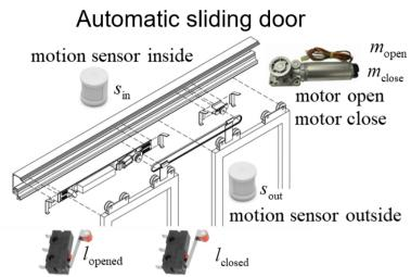
limit switch opened limit switch closed
