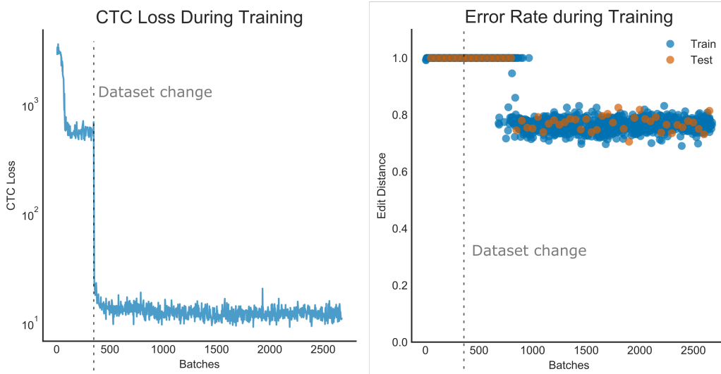
Figure 3: Results from training. To the left, CTC loss is shown. To the right, edit distance on the test set is shown. At Dataset change , both training and test set are changed from the spoken word set to the sung vocals dataset.
