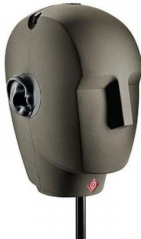
Figure 2: A Neumann KU 100 binaural recording device. A dense human like head contains two omnidirectional condenser microphones placed at a specific distance from each other to imitate the human ears. Realistic latex ears are placed outside the microphones, to imitate the filtering and localization effect of the human ears. (Taken from Neumann product catalog)
