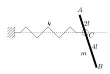
**Problem 2.** A thin homogeneous rod AB has mass m and length 6l. The point C, which is located 2l from the end point A, can slide smoothly along a horizontal line and rotate smoothly in a vertical plane. The point C is also attached to a horizontal linear spring with spring constant k = mg/l.
