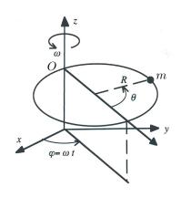
**Problem 2.** A circular, horizontal, ring of radius R is rotating with a given constant angular velocity  $\omega$  about a verical axis through the point O on the ring. On the ring, a small particle of mass m can slide smoothly. The position of the particle relative to the ring is given by the angle  $\theta$ . Derive the equation of motion for the particle (the differential equation for  $\theta$ ). Is it possible to have a motion with constant  $\theta$ ?
