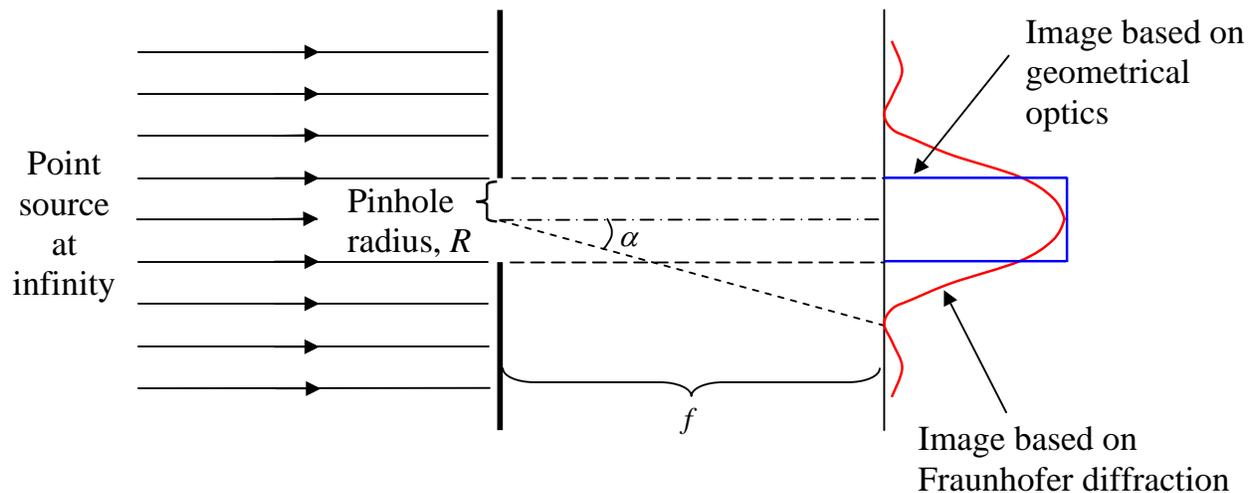
The image of a point object, the Point Spread Function (PSF), should be as small as possible to produce a sharp image.
