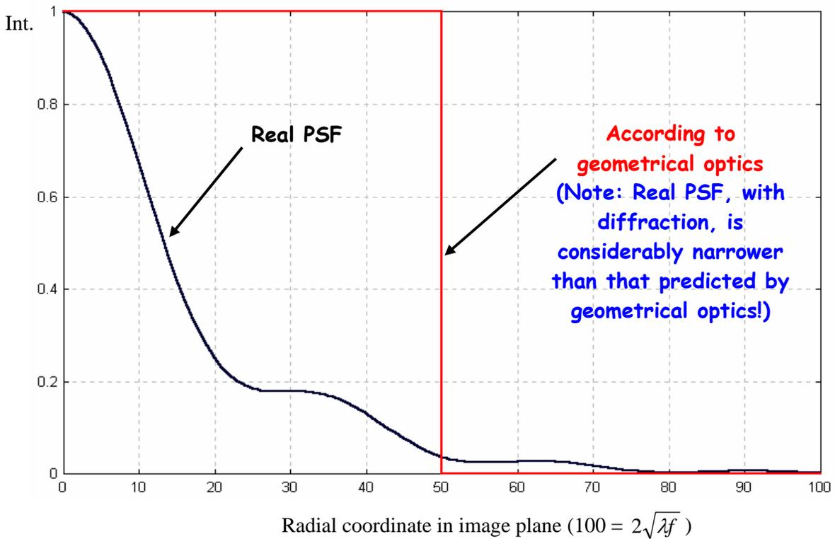
Full width of PSF at 37% intensity level (corresponds to resolution acc. to Rayleigh for small apertures)
