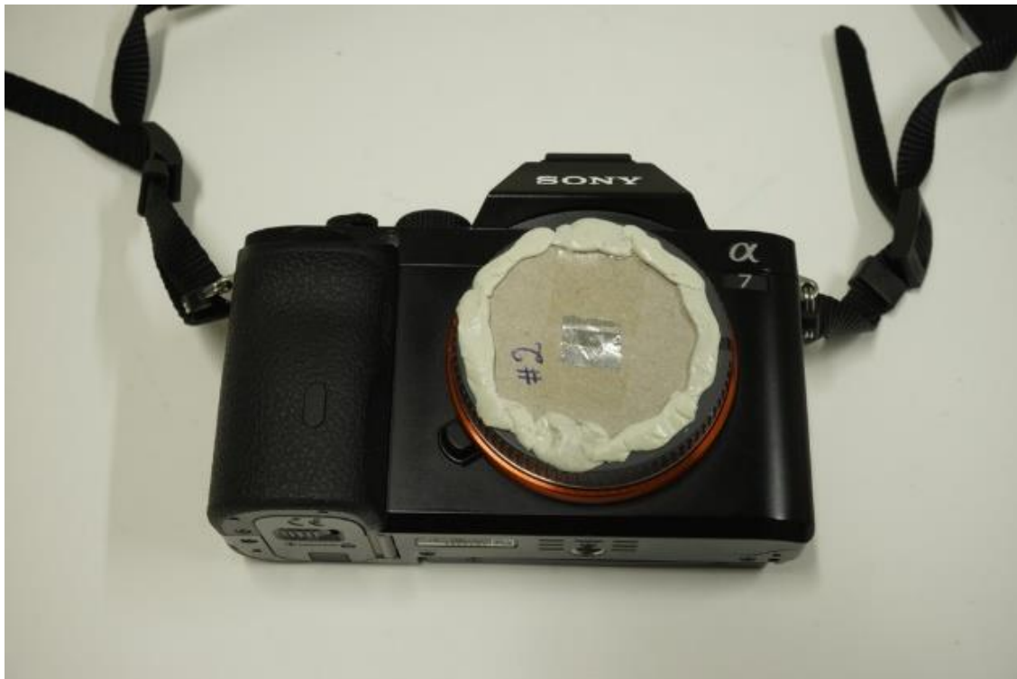
Sony A7 converted to pinhole camera. "Sticky tack" was used to attach to the camera body a piece of cardboard with an Al foil having a 0.2 mm hole in the center. Not so neat, but it works and stray light is blocked!
