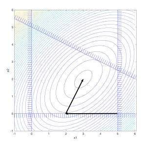
At the first iteration constraint 2 is in the working set. The direction points at  $(2\ 0)^T$ , which is feasible. Constraint 2 has a negative multiplier, -3, and it is hence deleted. The direction points at  $(3\ 2)$  which is feasible. No constraints are active, and we have found the optimal solution.
