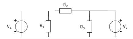
3. Determine the current I<sub>2</sub>.  $V_1$ =4 V,  $R_1$ =10  $k\Omega$  and  $R_2$ =30  $k\Omega$ .
