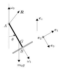
Use a basis triad with  $e_3$  in the  $r_{AB}$  direction and  $e_2$  horizontal. For the considered motion the angular velocity of the triad is
