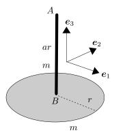
By continuous rotation symmetry, the symmetry axis is a principal axis and so is any perpendicular axis. Take the 3-axis to be along the symmetry axis.
