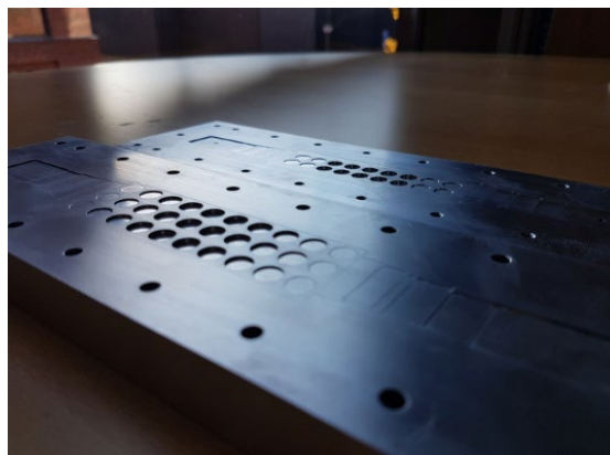
Glide-symmetric Luneburg lens antenna Filter designed at KTH in collaboration with Ericsson AB and European Space Agency.
