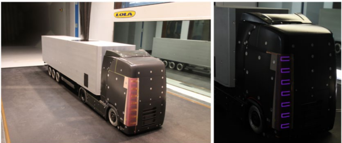
1:6 scale model of a truck in a wind tunnel: a) the right A-pillar is equipped with plasma actuator. b) a close-up of the actuators under actuation, the violet light show the plasma, experiments by Vernet, KTH (2017)
