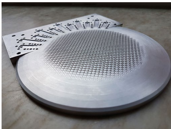
Glide-symmetric Luneburg lens antenna Filter designed at KTH in collaboration with Ericsson AB and European Space Agency.
