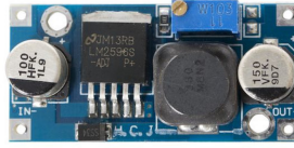
FIGURE C.2: Switched Variable Voltage Regulator, LM2596 from Luxorparts.
