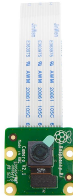
FIGURE C.8: The PiCamera Module.
