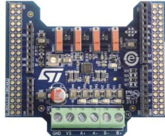
FIGURE C.10: Stepper motor driver, X-NUCLEO-IHM14A1 from Nu- cleo.
