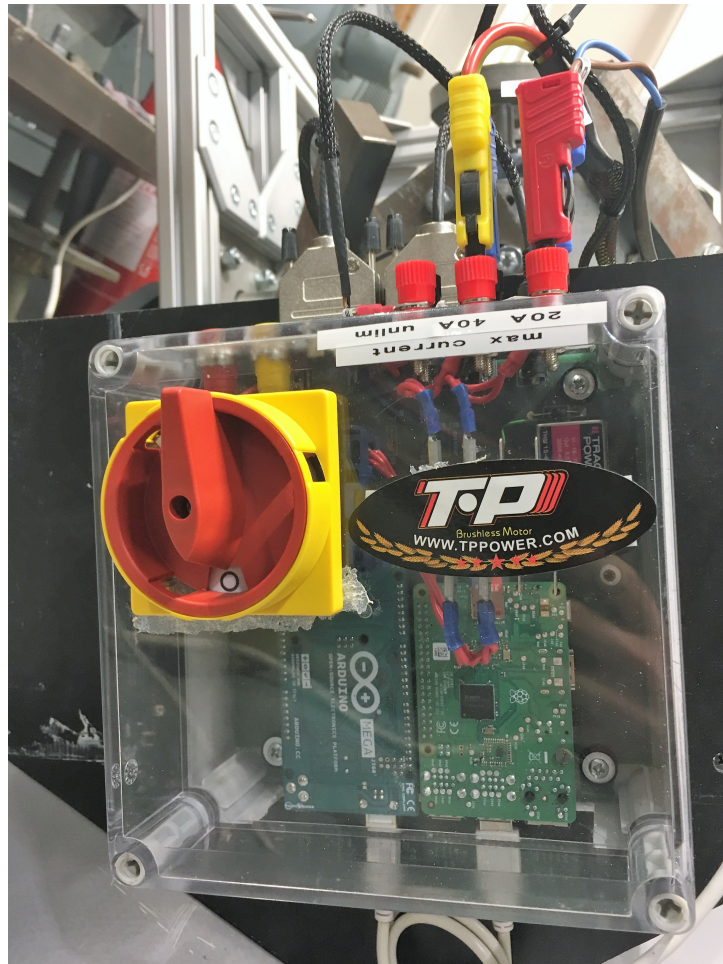
Figure 4.16: The closed control-box with main switch and power in and outlets at the top side.
