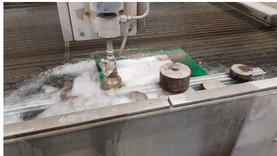
Figure 9: Extrusions cut to size using a water jet with help from KTH Prototype centre
