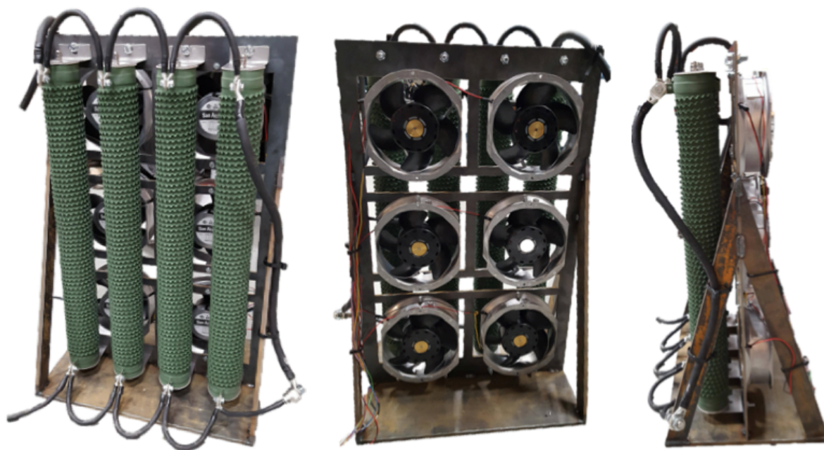
Figure 4.12: Picture of power resistor mount, from all three views.
