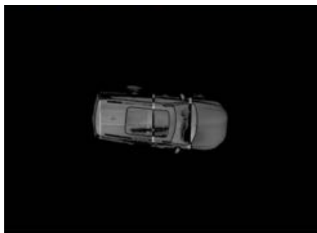
Figure 5.13: The segmentation is masked with a global threshold to reduce noise
