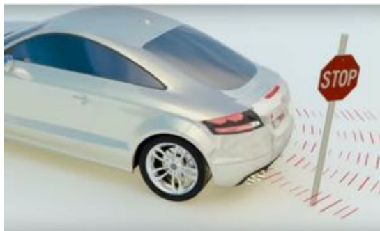
Figure 2.18: Narrow objects can fall in between the blind spots of the ultrasonic sensors. Normally a bumper contains six to eight sensors. Source: Video [3]
