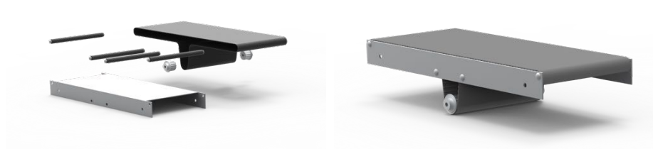
Figure 3.9: Conveyor belt design for station 1.
