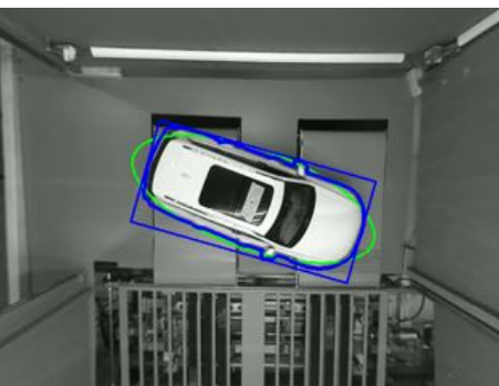
Figure 5.22: Comparison between fitEllipse (green) and minAreaRect (blue) for contour enfolding.
