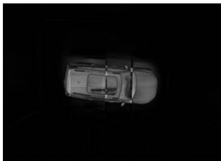
Figure 5.12: The difference between the blurred frame and the blurred reference image
