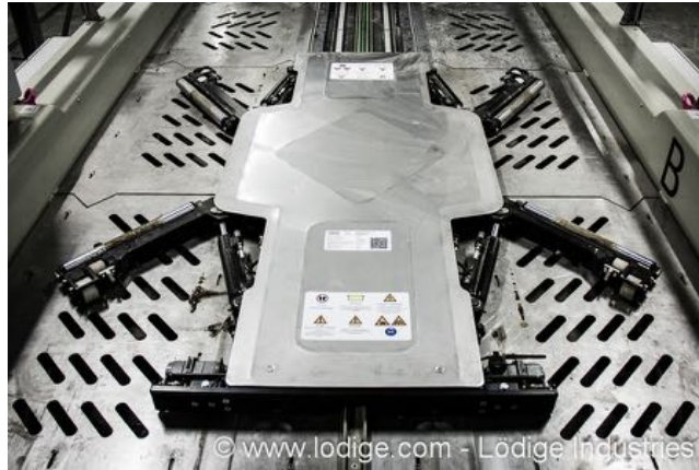
Figure 2.9: Non-pallet solution with carts lifting the wheels of the car by unfolding two arms under each wheel. Source: Lödige Industries
