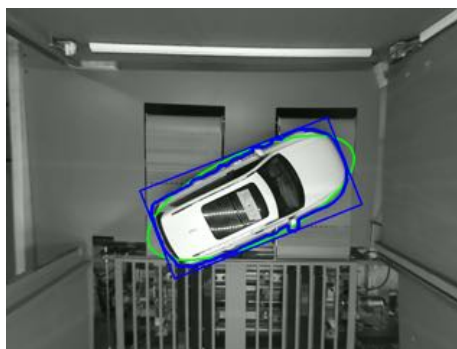
Figure 5.22: Comparison between fitEllipse (green) and minAreaRect (blue) for contour enfolding.
