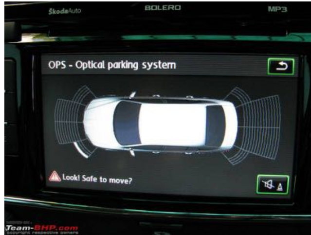
Figure 2.16: The graphical interface for a type of proximity sensor system. Source: Team-BHP.com
