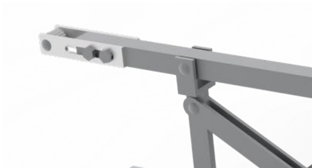
Figure 3.16: Tensioning mechanism for side belts
