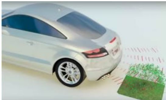
Figure 2.19: Ultrasonic sensors have a difficulty detecting inclined or poorly reflective objects. Source: Video [3]
