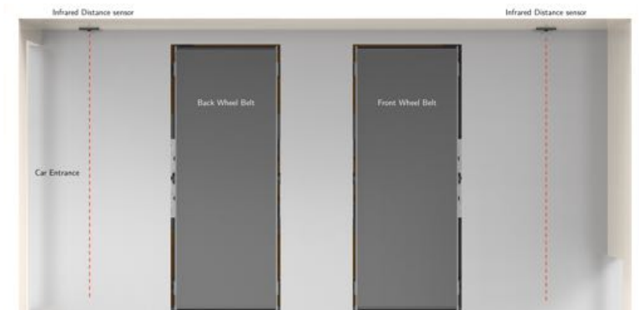
Figure 4.4: Illustration of the position of the two IR sensors.
