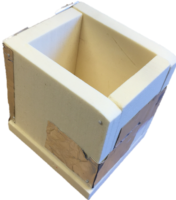
Figure 4.2: Box made of the mentioned sandwich construction to test the heat resistance
