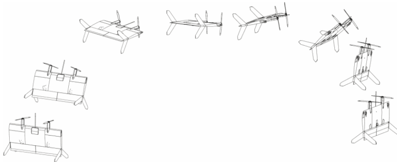
Figure 14: Hover, level, and transition of Wingtra
