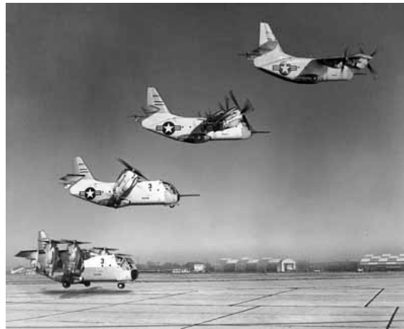
Figure 12: The transition from VTOL to horizontal flight by the LTV-Ryan-Hiller [30].
