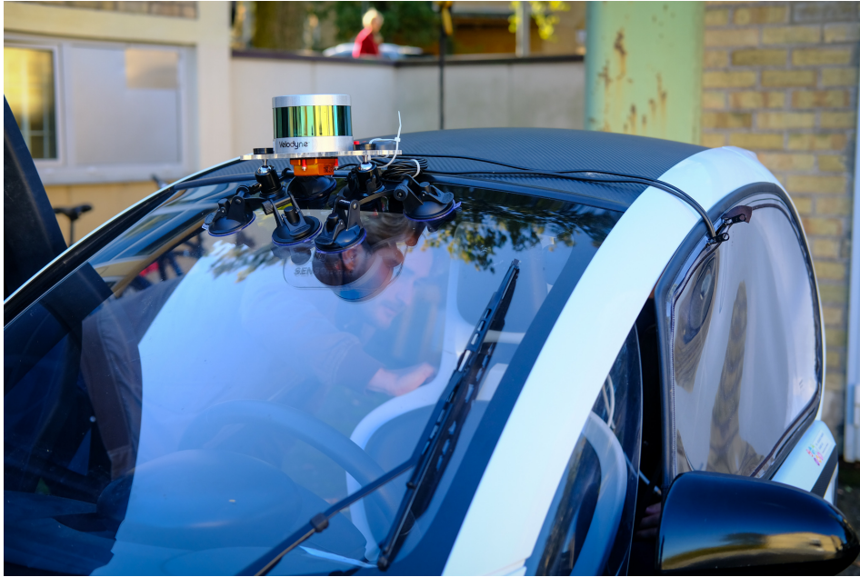
Figure 5.2. The sensor rig mounted on the Renault Twizy, with cables drawn into the car through the driver's window.
