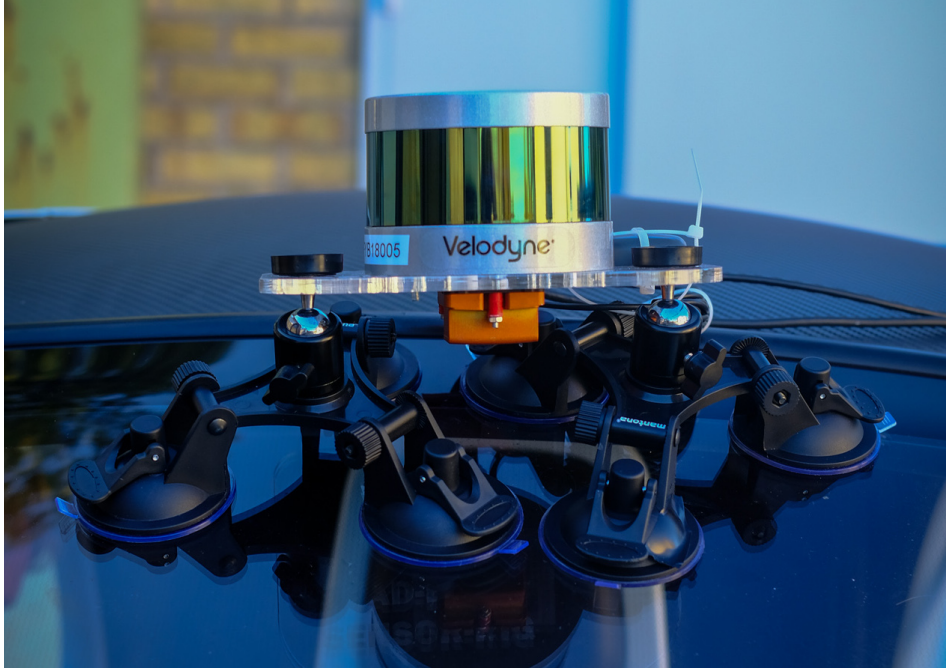
Figure 5.1. Close up of the sensor rig with Lidar on top and IMU underneath.
