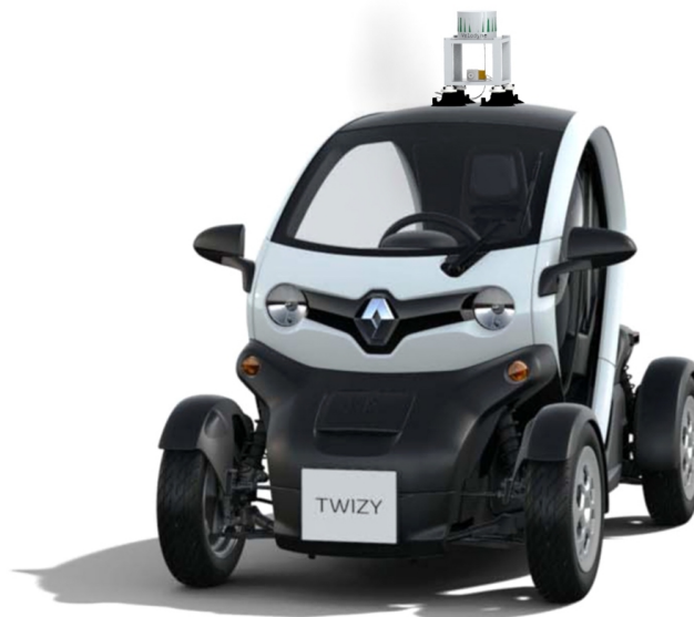
Figure 3.2. Sensor rig mounted on a Renault Twizy. Generated with Solid Edge and rendered in Keyshot.
