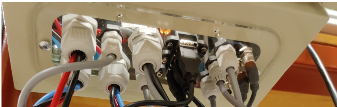
Figure 49: Cable interface on the electrical cabinet
