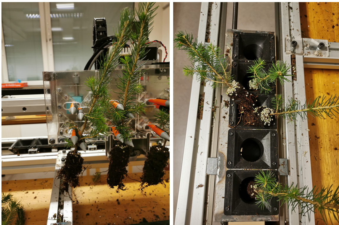
(a) Seedling askew due to only being gripped with 2 (b) Two seedlings in one buffer cup due to tilted plant fingers
