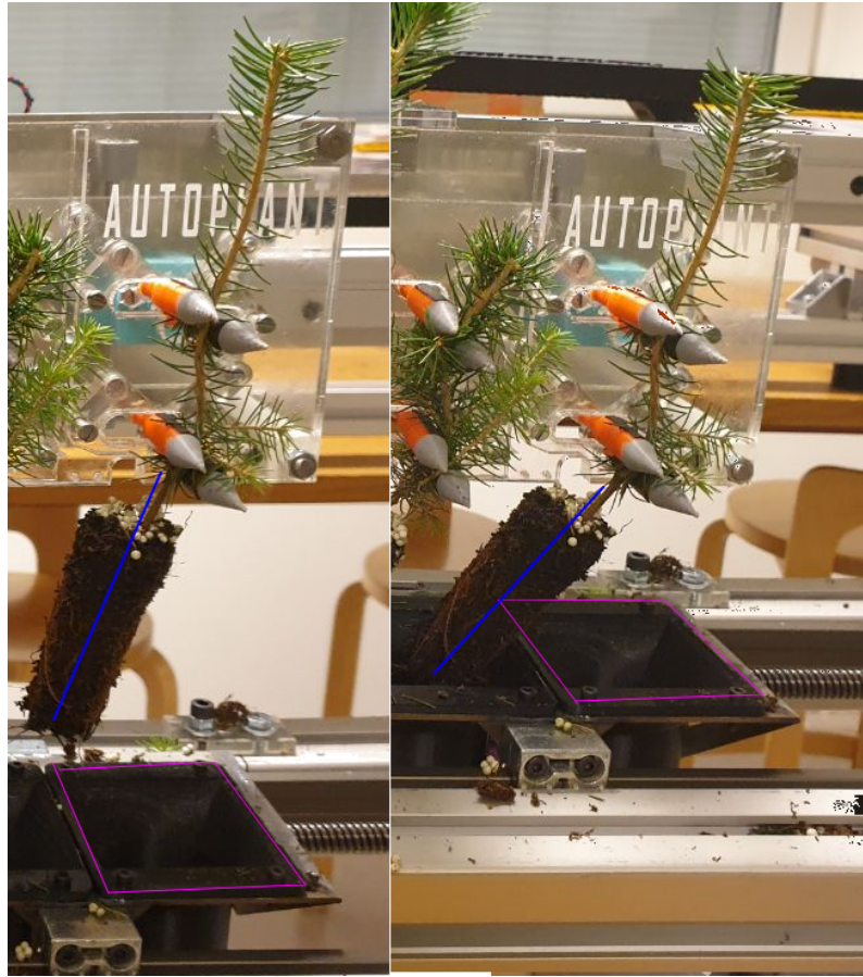
Figure 81: A problem encountered with the gripper subsystem were tilted seedlings when gripped. This would cause failure in inserting the seedlings into the buffer system cups appropriately. The pink outline highlights the buffer cup opening the seedling was supposed to be inserted into. The tilt of the seedling is highlighted by the blue line.
