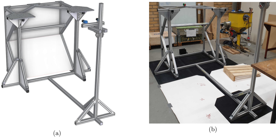
Figure 5.2: Side by side comparison between the CAD design and the real life implementation of the rig.
