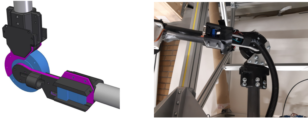
Figure 5.5: Side by side comparison between the CAD design and the real life implementation of the Elbow for both arms.
