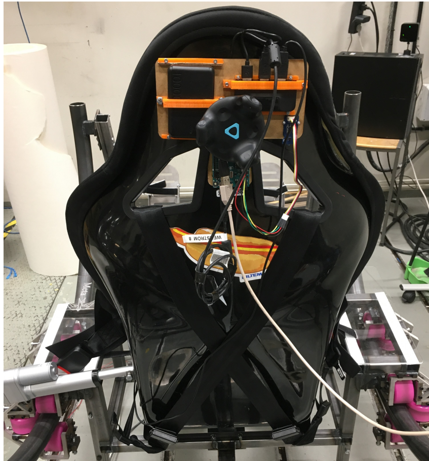
Figure 4.20: The electronic plate mounted on the chair with all the components.
