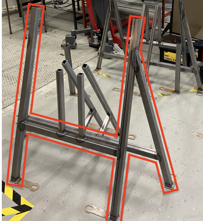
Figure 4.2: The parts that make up the main frame are encircled in red.
