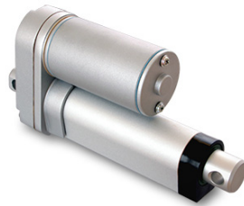
Figure 3.32: Linear motor, 12 VDC, 250 N and 2.4 A. [41]
