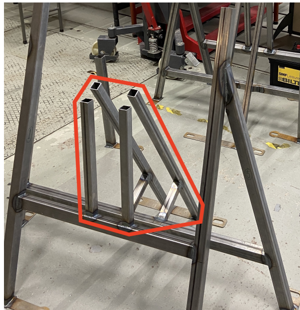
Figure 4.4: The parts that made up the pulley frame are encircled in red.
