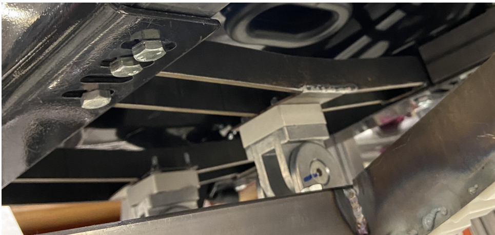
Figure 4.13: The support beams that connect the chair to the roll axles.
