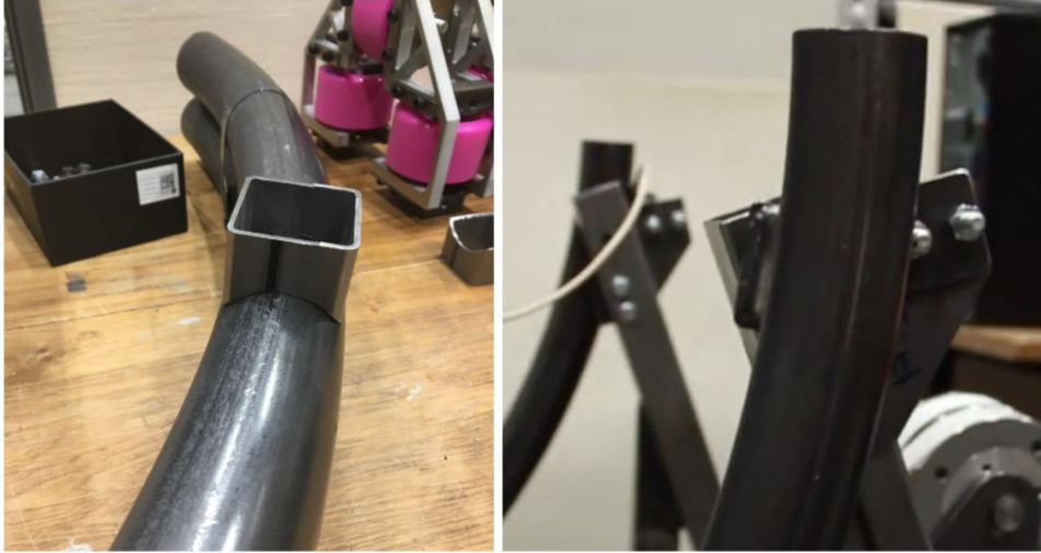
Figure 4.3: The mounts where the curved rails are attached to the frame.
