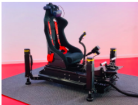
Figure 2.19: Generic Airplane Simulator (pitch, roll and heave), $21 369 [34].
