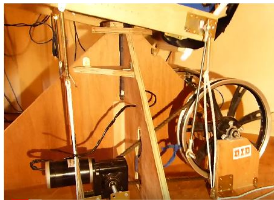
Figure 2.14: Improved version with a gear attached between the motor and the rod [28].
