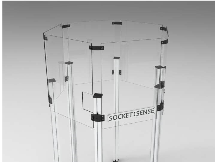
Figure 5.8: Render of the final Design, made in Solid Edge. Demonstrates the protective layer of acrylic sheets.
