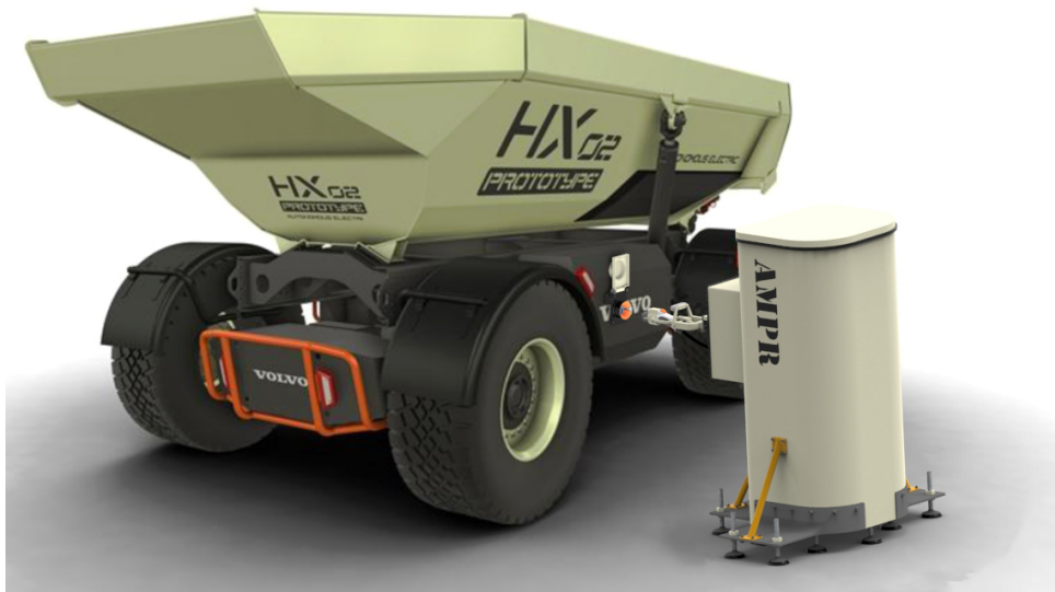
Figure 34: Complete design of the system. Charging station and lid made in Solid Edge. Carrier is from Volvo [23].
