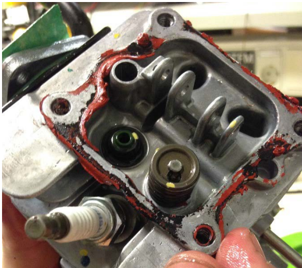
Figure 8. Valve position in the cylinder head of the Honda GXV 57
