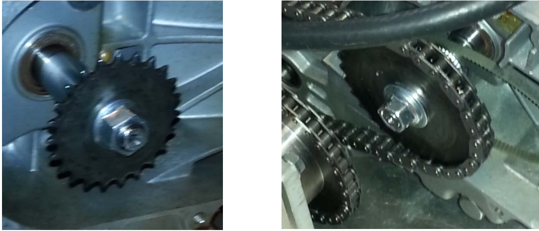
Figure 13. Two sprockets made for the new engine. Left: Sprocket connecting ICE to electric motor on the test rig. Right: Sprocket connecting ICE to drivetrain in vehicle with chain
