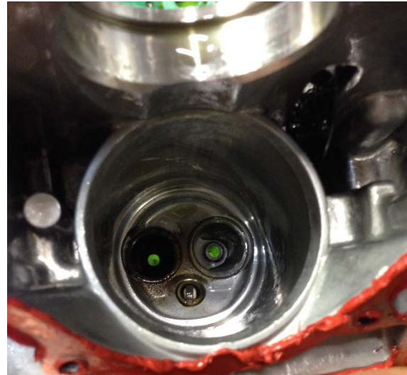
Figure 8. Valve position in the cylinder head of the Honda GXV 57
