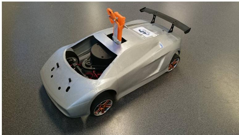
Figure 37: The original chassis was altered to suit the car and painted in a gray nuance.
