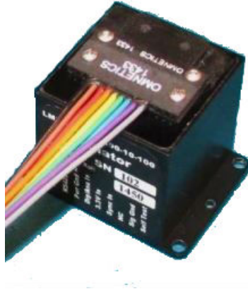
Figure 3.32: G200D-100-300 digital triaxial gyro
