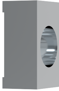
Figure 3.18: Clamp to push the rail towards its reference.
