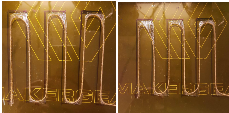
Figure 31: To the left: the thread is fed at 271.8 mm/min. To the right: the thread is fed at 362.4 mm/min
