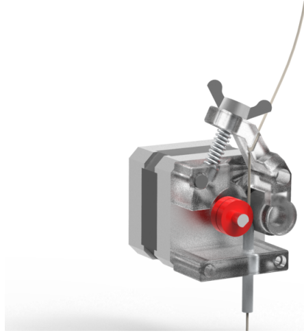
Figure 16: The thread is fed by rollers controlled by a stepper motor
