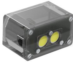
Figure 2.25: The first design of the LED case, with PCB and screws attached.
