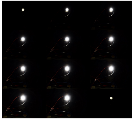
Figure 2.8: Results from PWM verification. Photos of PWM-dutycycle 0, 10, 20,...,100%.
